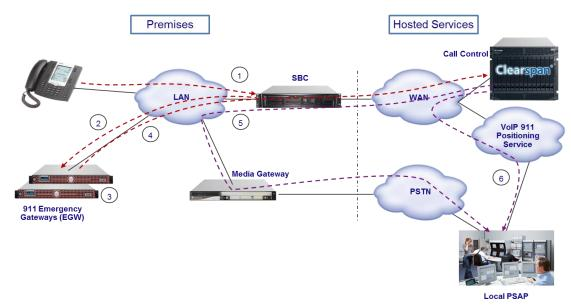
Figure 22. Advanced Clearspan E911 Call Flow for Normal Operation.
