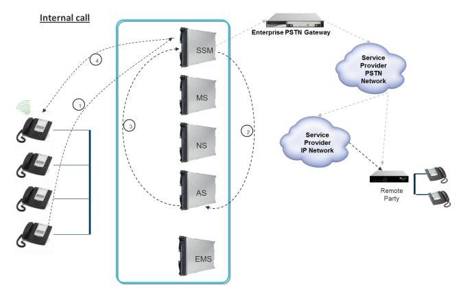
Figure 20. Internal Call setup Call Flows.
