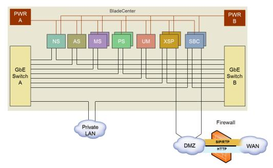
Figure 11. Typical High-level BladeCenter Architecture.
