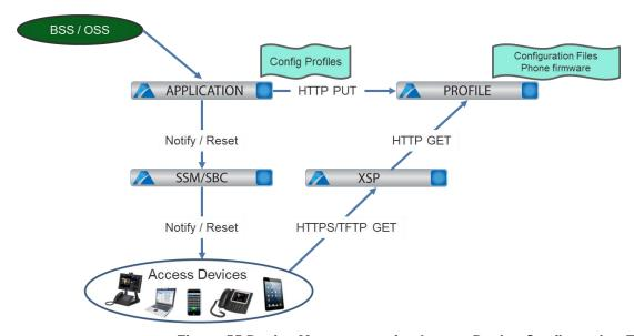
Figure 55 Device Management for Access Device Configuration Files.
