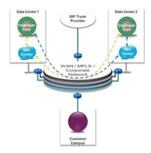
Figure 12. SBC Cross Coupling.
