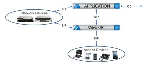
Figure 4. CORE SBC Platform Interaction.
