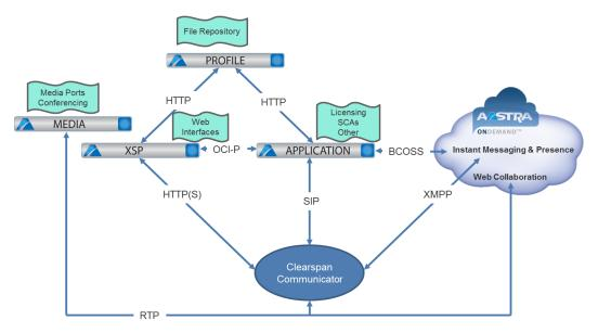
Figure 23. Clearspan UC High-level Architecture.
