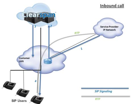
Figure 17. Clearspan Inbound Signaling and Call Flows.
