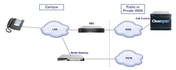
Figure 14. Simplified Remote Campus Architecture.
