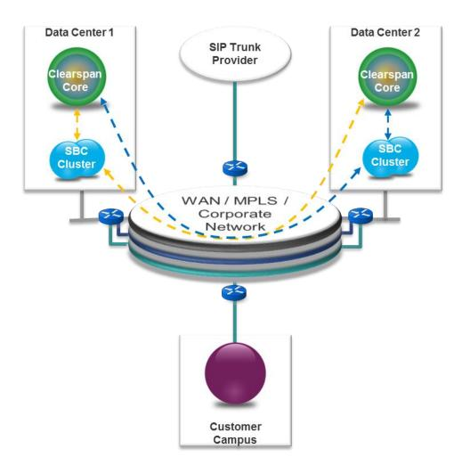
Figure 1. High-Level Clearspan Architecture.
