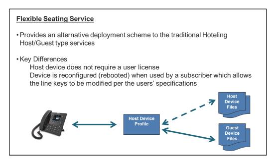
Figure 37. Clearspan Flexible Seating service.
