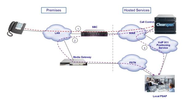
Figure 21. Basic Clearspan E911 Call Flow for Normal Operation.
