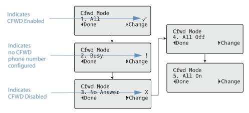
In this example, **CFWD All** is enabled as indicated by a check mark  $(\checkmark)$ , **CFWD Busy** is enabled but no call forward phone number is configured as indicated by a !, and CFWD No Answer is disabled, as indicated by an X.
